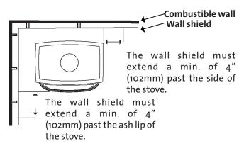
Must be 1" off the wall and 1" off the floor. With standard legs, the shield must be 40" high. With optional short legs, the shield must be 38" high. Both shields must extend and join in the corner.
